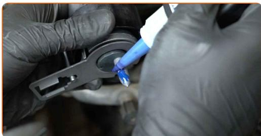
**78** Paigaldage hammasrihma pingutusrull.
