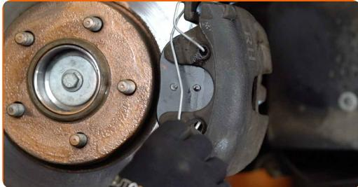
**Vahetamine: piduriklotside – FORD Focus Mk2 Hatchback (DA\_, HCP, DP).**
