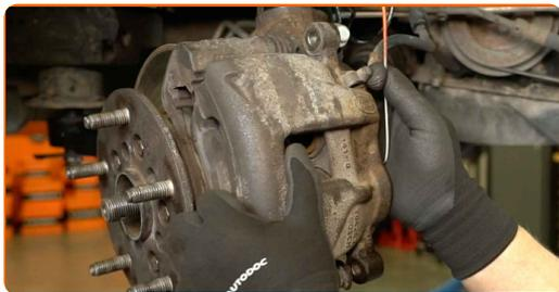
Vahetamine: piduriklotside – FORD Transit Mk6 Minibus (V347, V348).
