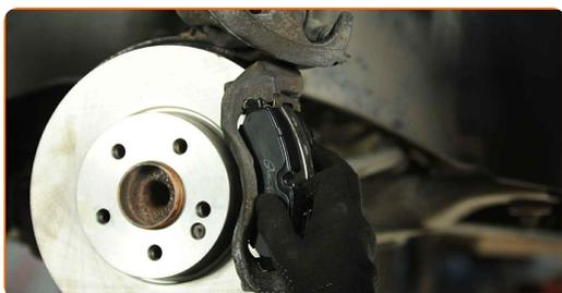
Vahetamine: piduriklotside – MERCEDES-BENZ SPRINTER 3-t Buss (906).
