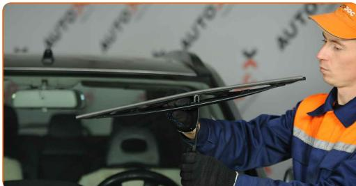
Vahetamine: klaasipuhastite – RENAULT Megane IV Hatchback (B9A/M/N\_).
