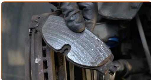
Vahetamine: piduriklotside – SKODA Octavia III Hatchback (5E3, NL3, NR3).
