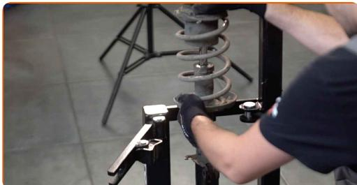
Vahetamine: vedru – VAUXHALL Corsa Mk II (C) Hatchback (X01).
