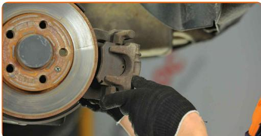
**Vahetamine: piduriketaste – VW New Beetle Hatchback (9C1, 1C1).**
