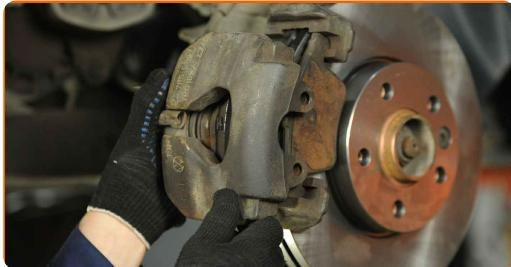
Vahetamine: piduriklotside – VW Transporter V Buss (7HB, 7HJ, 7EB, 7EJ, 7EF, 7EG, 7HF, 7EC). AUTODOC soovitab:
